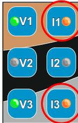
Current phases A & C may be swapped over OR possibly have very bad Power Factor due to excessive lagging current. In the latter case the phases may be correct.
