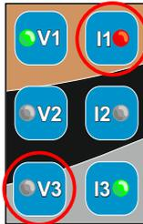
No signal received by CB phase voltage lead. Check connection.
