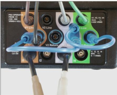
A successful hook-up (based on physical connections and corresponding instrument configuration) is demonstrated as follows:
