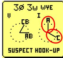
The CTs are on the wrong phases. Swap the CTs around to align voltage and current Phasing.
