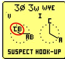
The CB voltage phase has a bad connection. Try reconnecting.
