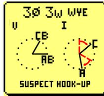
Power Factor is severely lagging (beyond 45°). "Suspect Hook-Up" message displayed. THIS MAY BE CORRECT so no solution needed.
