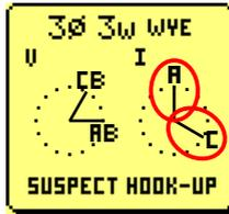
The CTs are on the wrong phases. Swap the CTs around to align voltage and current Phasing.
