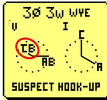
The CB voltage phase has a bad connection. Try reconnecting.
