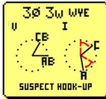
Power Factor is severely lagging (beyond 45°). "Suspect Hook-Up" message displayed. THIS MAY BE CORRECT so no solution needed.
