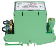
Example of a closed, toroid current clamp used (GF1).
